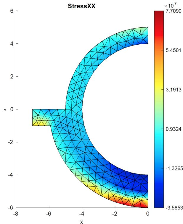
Figure 5.1: Stress in  $x$  direction when flange is supported at the bottom
