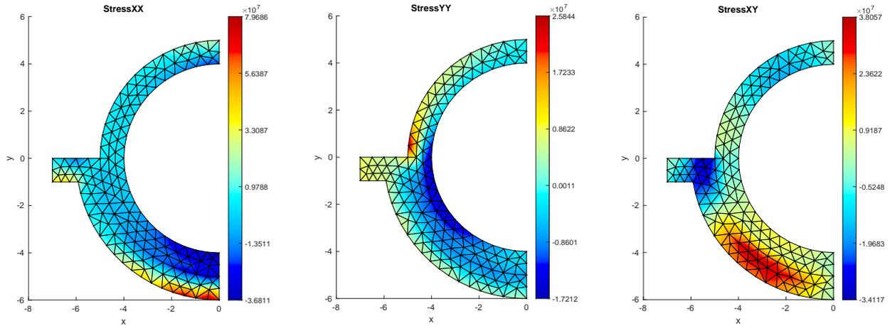
Figure 4.3: Stress distribution throughout flange and pipe
