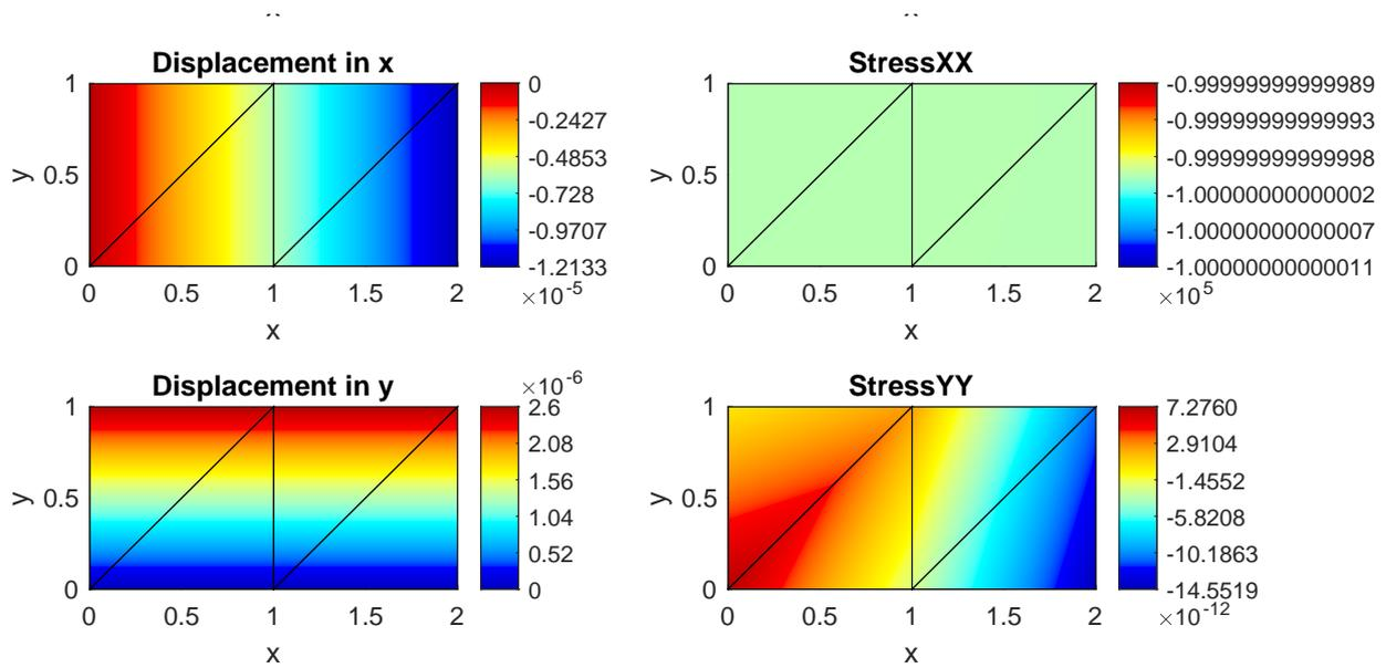
Figure 3.4: A pressure of 1 bar applied to the right edge
