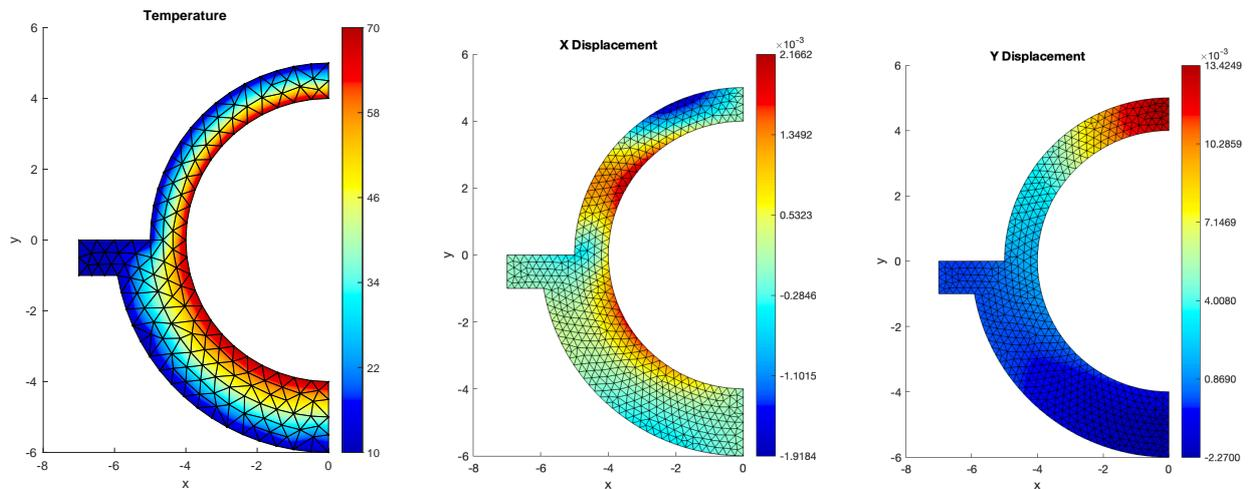
Figure 4.1: Temperature and displacement distributions throughout flange and pipe
