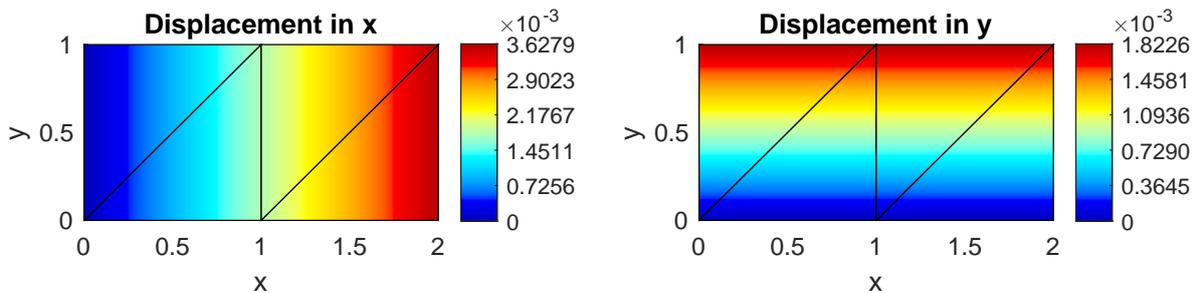
Figure 3.5: Combined displacements for temperature difference and pressure
