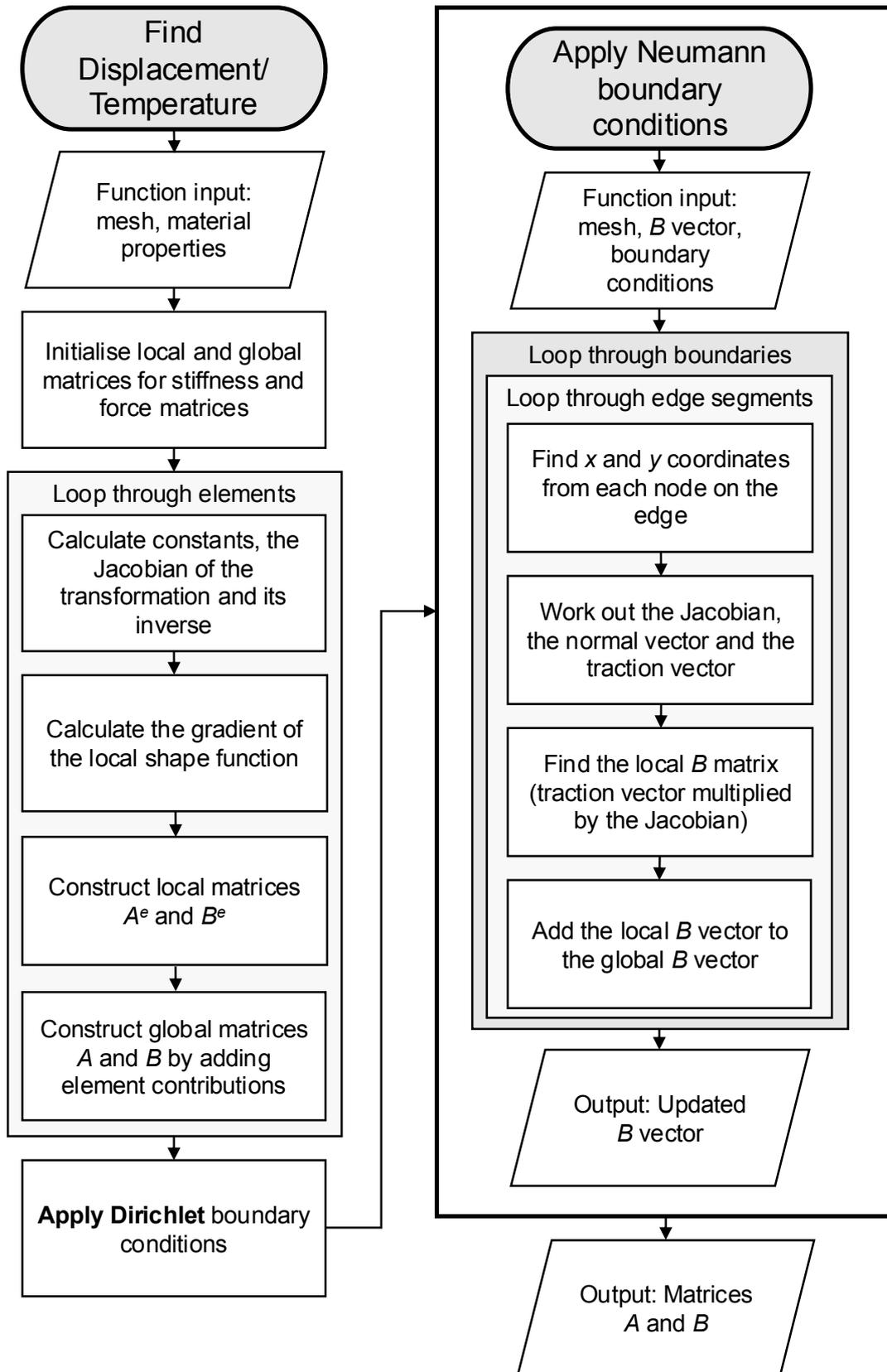
Figure 2.1: Flow chart for developing a finite element programme
